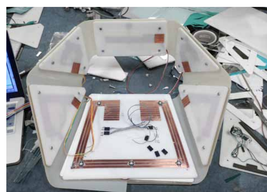
The six pads mounted on the flexible substrate during assembly of the prototype.
