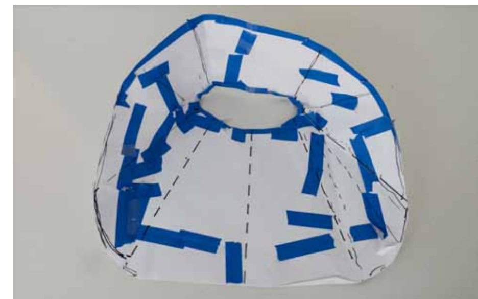
Tailor-made prototype consisting of paper patches for determining the form and size.
