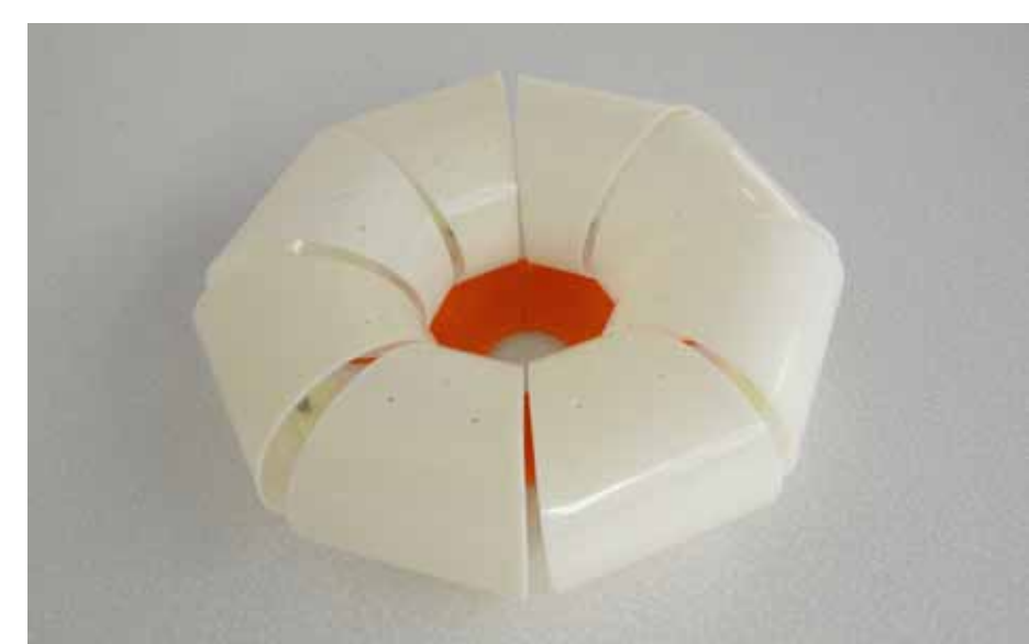
The torus (donut) concept consists of 8 pressure-sensing and illuminating components
