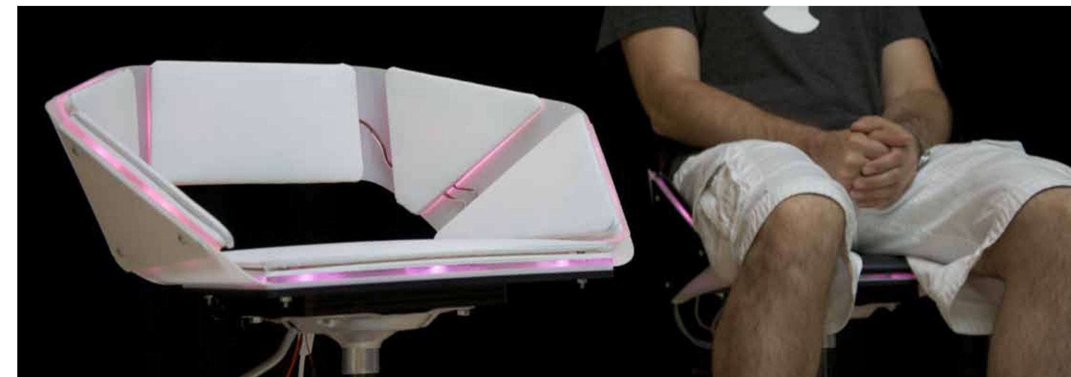
The measurements from the sensors of the black BodyPod in the background (far right) are mapped through color and light to the corresponding pads of the white BodyPod in the foreground (left).
