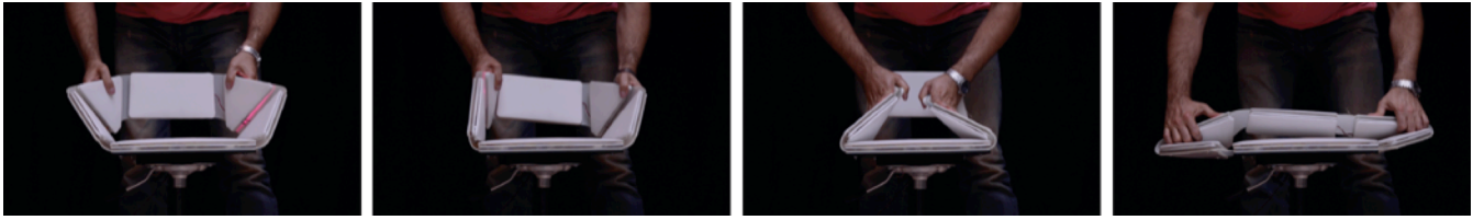
Figure 5. Each BodyPod consists of a flexible surface with six pressure-sensing and light-emitting pads that can deform and fold.
