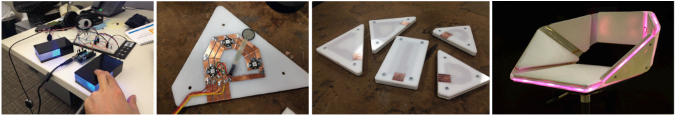
Figure 4. Building the pressure sensing and lighting in the pads. From left to right: early prototype “bricks” to experiment with lighting behavior; wiring inside a pad; assembled pads; mounted pads with cushions on the Nylon chair form.
