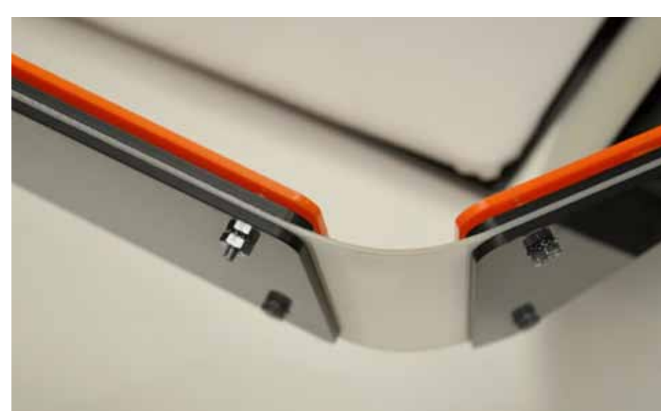
Detail of the assembly showing the flexible Nylon sheet and the rigid Delrin pads.
