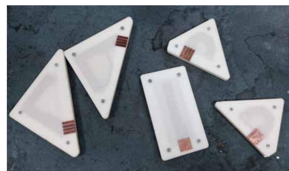
The 6 pressure-sensing pads
